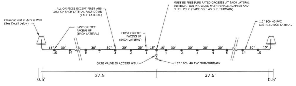
1/8" Orifices with Orifice Shields
